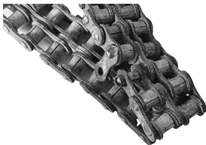
Corrosion of Stainless Steel Drive Chain
