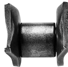
3) Offset Link Plate Fatigue Offset link plates are bent at the center, and the resulting concentration of stress at the bend can cause a fatigue break. Avoid using offset links in high-pressure applications.
