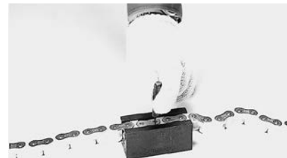
Figure 16: Disconnecting Poly Steel Chain
