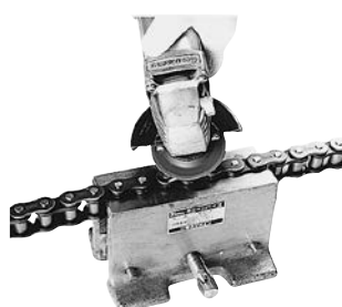
Figure 7: Grinding Down Pin Ends
